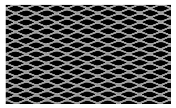
LW Aperture:14.22mmStrand Width:1.80mmSW Aperture:4.80mmThickness:0.70mmWeight:2.40 kg / m2Open Area:57%
